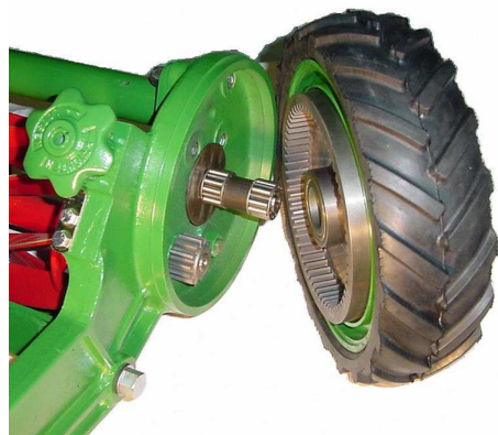
Cast Iron Wheels with Machined Gears
